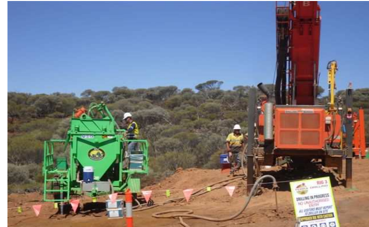
No sumps – fully enclosed system
