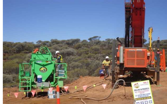
No sumps – fully enclosed system
