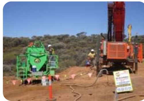
No sumps – fully enclosed system
